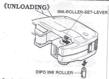
Turn the right side of the body downward and push the INK-ROLLER-SET-LEVER to the arrow direction for the DIPO INK ROLLER to slip out of the hole.
